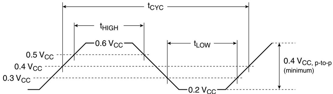
**Signal Timing Parameters**
