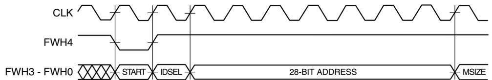
**START:** This one-clock field indicates the start of a cycle. It is valid on the last clock that FWH4 is sampled low. The two start fields that are used for the cycle are shown in Table 3. If the start field that is sampled is not one of these values, then the cycle attempted is not an FWH memory cycle. It may be a valid memory cycle that the FWH component may wish to decode, i.e., it may be of the LPC memory cycle variety.
