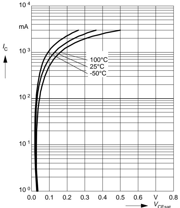
**Collector current  $I_C = f(V_{BE})$**
