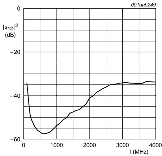
$I_S = 4.3 \text{ mA}$ ;  $V_S = 5 \text{ V}$ ;  $P_D = -35 \text{ dBm}$ ;  $Z_o = 50 \Omega$ .
