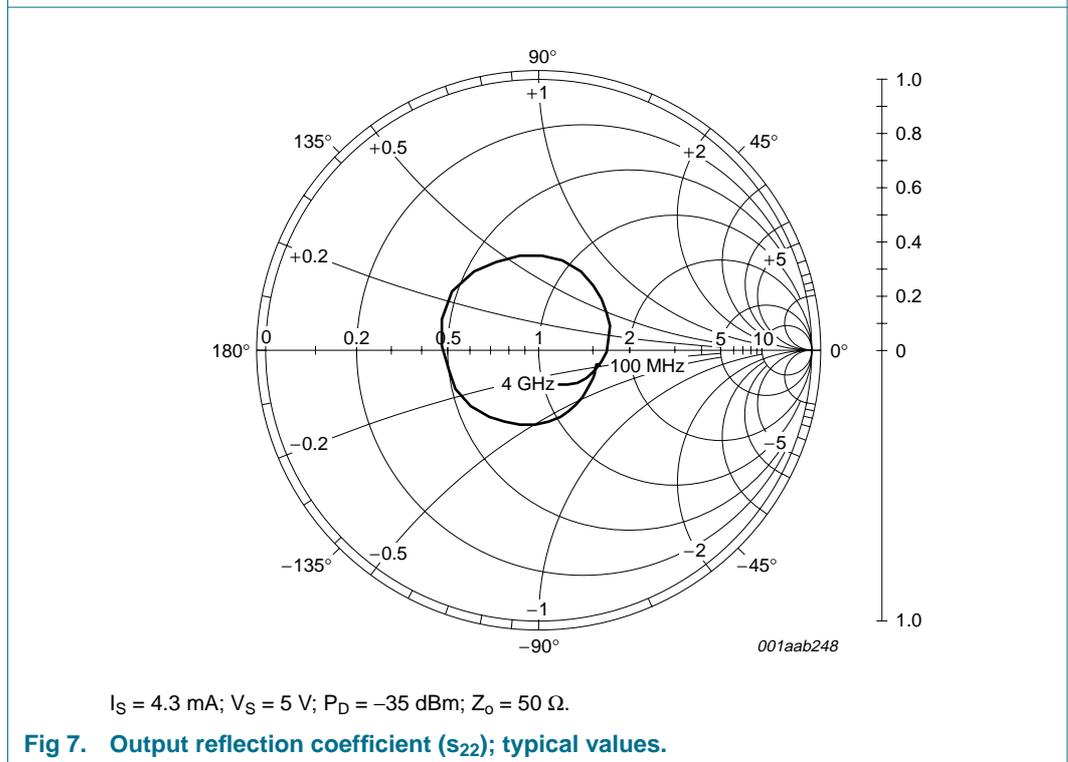
$I_S = 4.3 \text{ mA}$ ;  $V_S = 5 \text{ V}$ ;  $P_D = -35 \text{ dBm}$ ;  $Z_0 = 50 \Omega$ .
