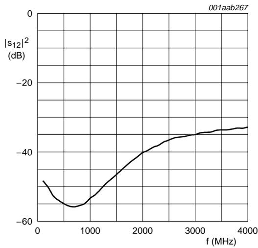
$I_S = 8 \text{ mA}; V_S = 5 \text{ V}; P_D = -35 \text{ dBm}; Z_o = 50 \Omega.$
