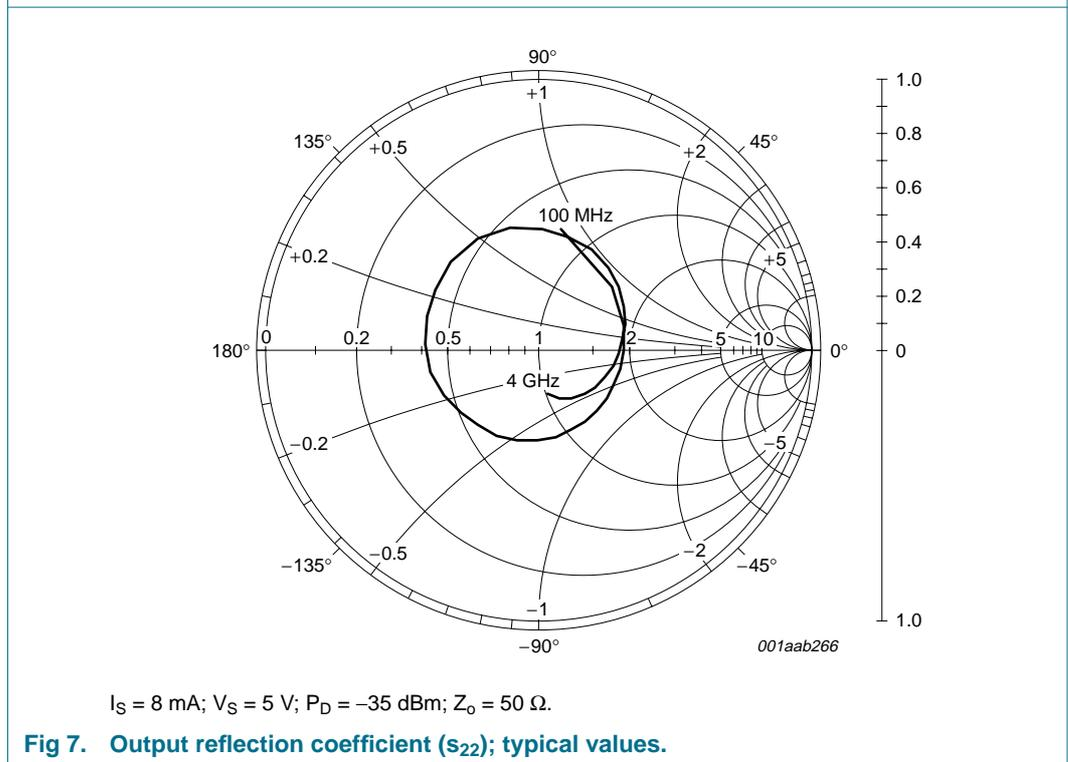
$I_S = 8 \text{ mA}$ ;  $V_S = 5 \text{ V}$ ;  $P_D = -35 \text{ dBm}$ ;  $Z_o = 50 \Omega$ .
