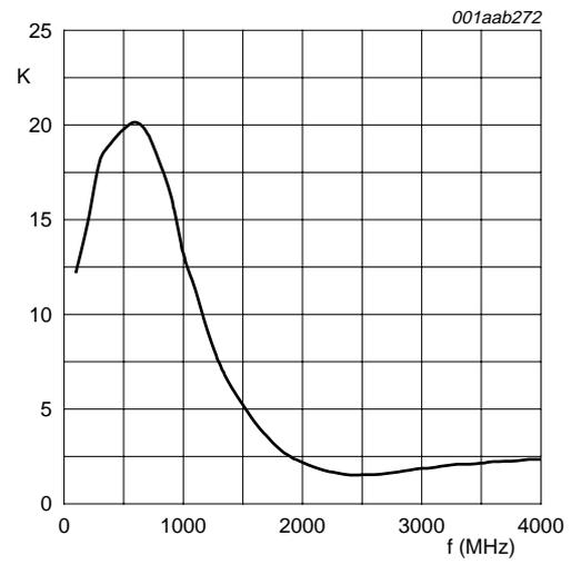
$I_S = 8 \text{ mA}$ ;  $V_S = 5 \text{ V}$ ;  $Z_o = 50 \Omega$ .
