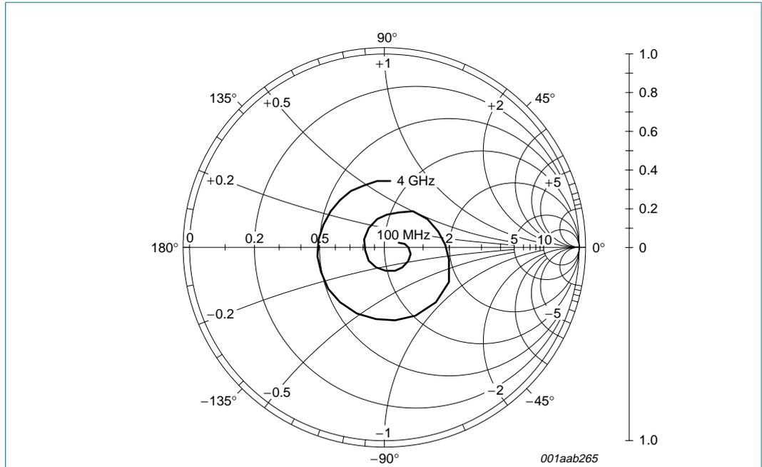
$I_S = 8 \text{ mA}$ ;  $V_S = 5 \text{ V}$ ;  $P_D = -35 \text{ dBm}$ ;  $Z_o = 50 \Omega$ .
