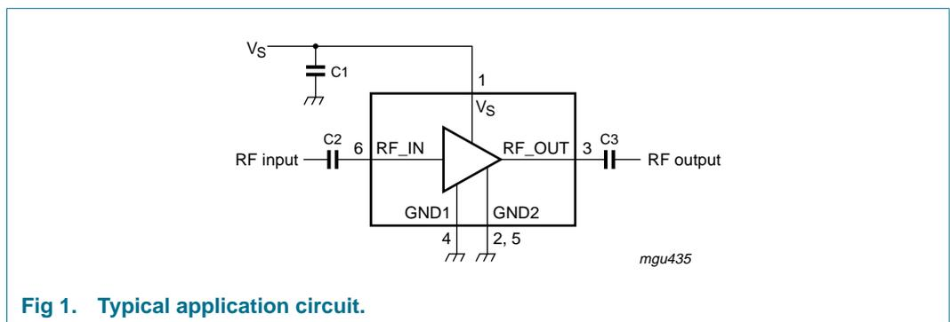
**Fig 1. Typical application circuit.**
